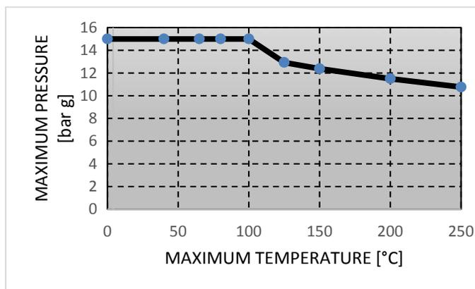
**However, if the filter is used at temperatures above 100 °C contact Asco Filtri.**
