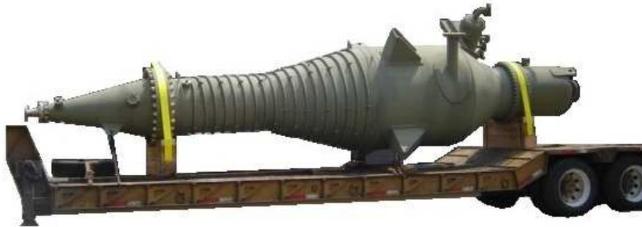
The Mott **HyPulse GSP** is a traditional filtration system for process gas and steam, suitable for all applications where working conditions prevent the use of cyclones or bag houses. When the pre-set Delta-P is reached or by timing, the gas feed is stopped, the filter isolated and filter cleaning takes place by flow inversion.
