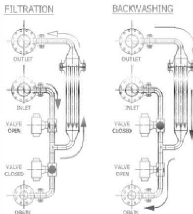
In case of modular filtration system with external fluid back-wash, the feed fluid is distributed from inlet header to the stations; the automatic feed and the outlet valves are open while the automatic drain and the back-wash fluid feed valves are closed.
