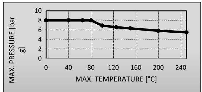
**However, if the filter is used at temperatures above 80 °C contact Asco Filtri.**
